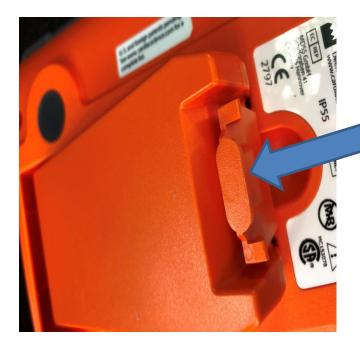
You will find the battery on the back of the defibrillator. To change the battery on the G5 defibrillator squeeze the tab indicated towards the battery and then remove from device. To replace put the non-tab end of the battery into the device first then push the battery into the defibrillator.
