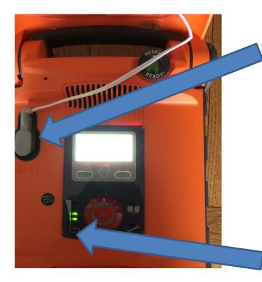
This is the pads connected to the defibrillator and ready to use. To replace the pads simply pull upwards on the grey plug and replace with the spare set in the back of the case by simply pushing the grey plug of the new pads into the socket.
